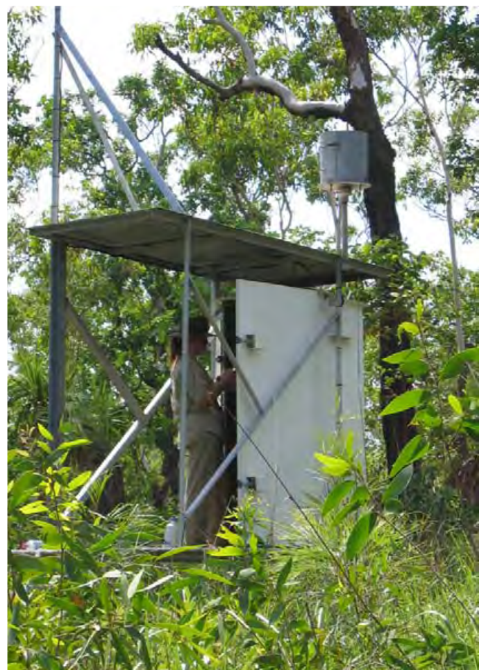
Water quality samples and flow data are collected at a gauge station.
