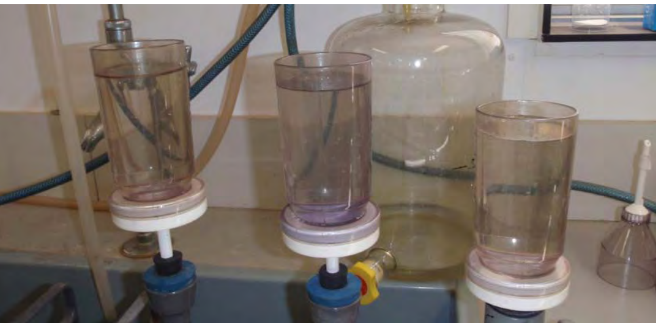
Laboratory equipment used to filter chlorophyll a water samples.
