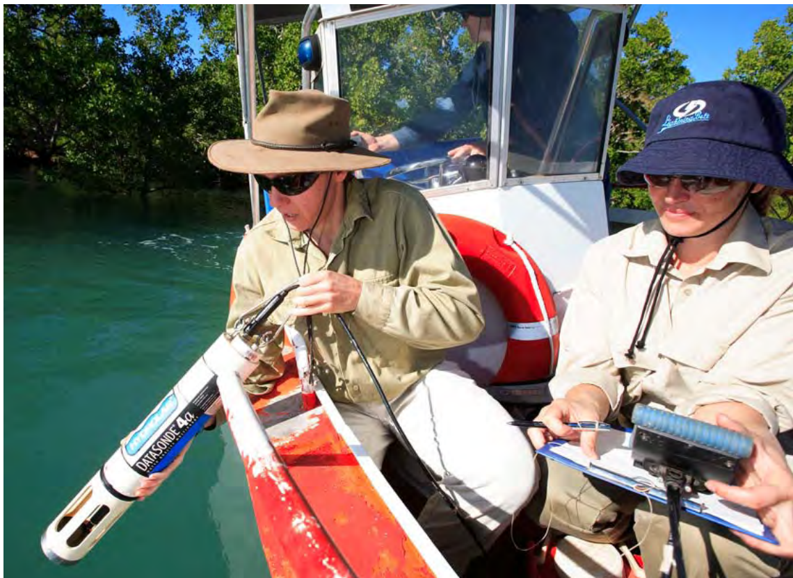
A Hydrolab datasonde is used to measure water quality indicators.
