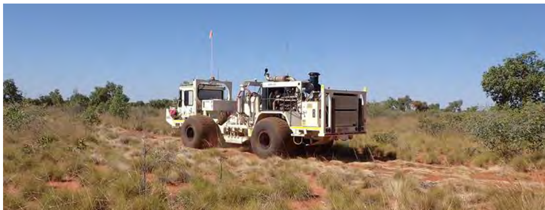
Figure 11: Example of a vibroseis truck used during seismic acquisition
