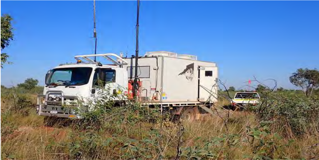
Figure 12: Data recording van used during seismic acquisition
