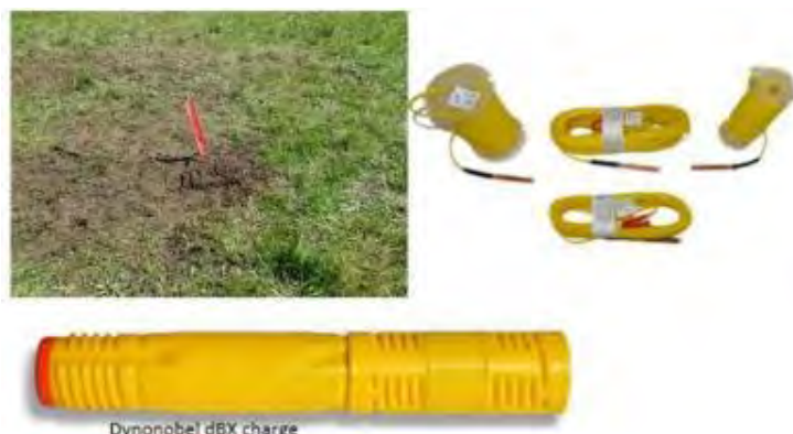
Figure 10: Example of loaded charge in hole ready for detonation and example of a charge used in seismic survey acquisition; charge length is approximately 400 – 500 mm
