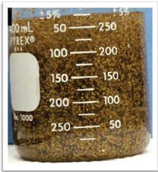
Figure: Typical sand - guar gum fluid mix. (Source Economides and Martin, 2007)
