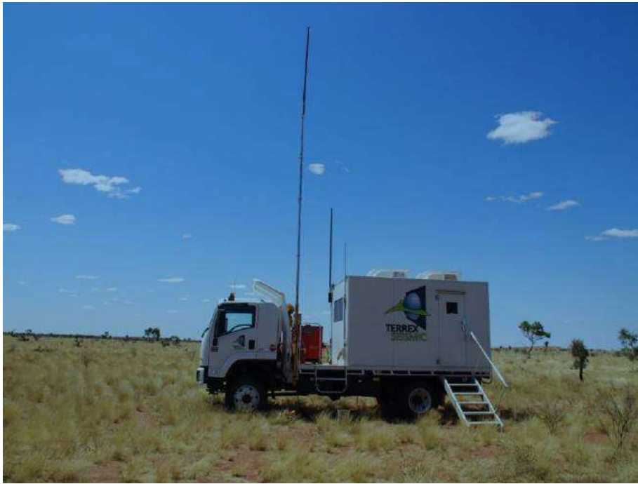
Figure: Seismic Recording Truck
