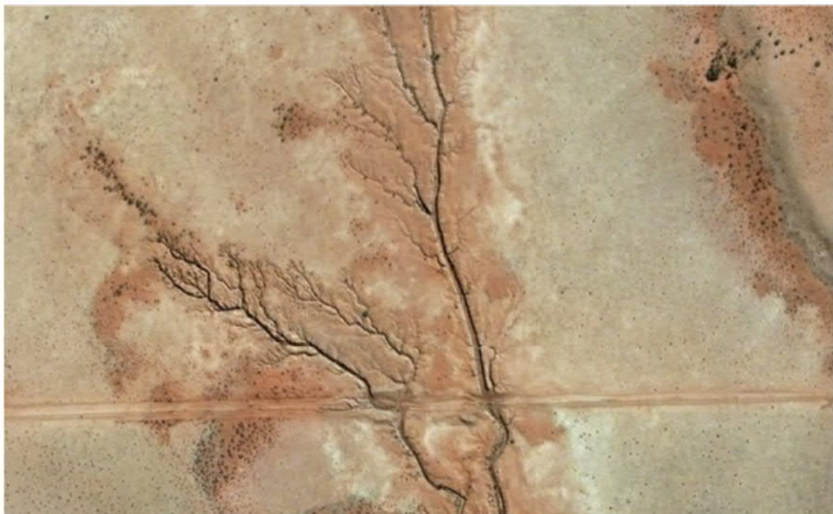
Figure 3-6. Close up of erosion of Track section B (western most dot on Figure 3.4)
