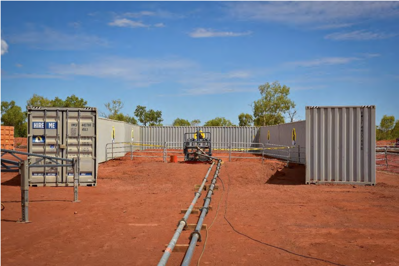
Figure 29: Horizontal flare set-up (Note: the pit has a coletanche liner located ~500mm below the surface)
