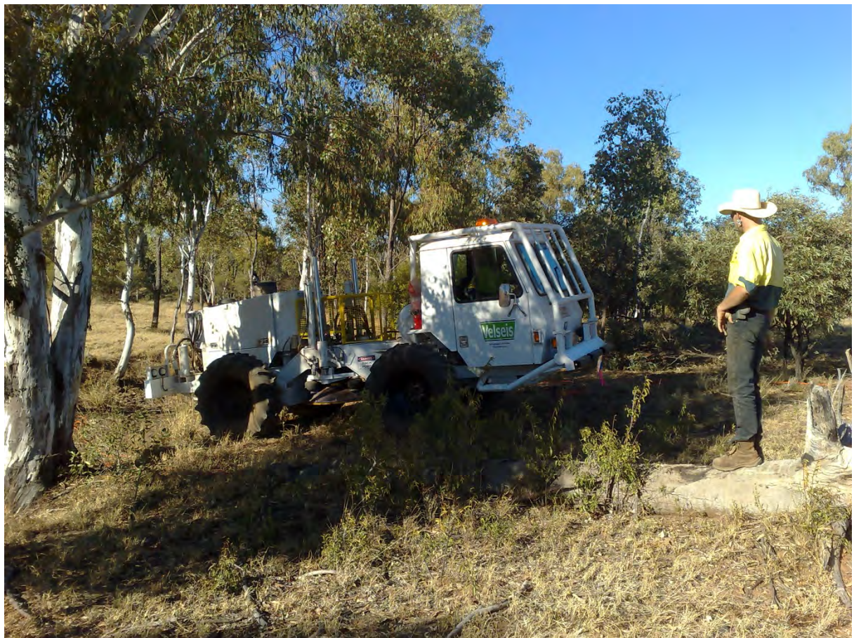
Figure 2.8: Vibroseis buggy traversing uncleared watercourse (a)
