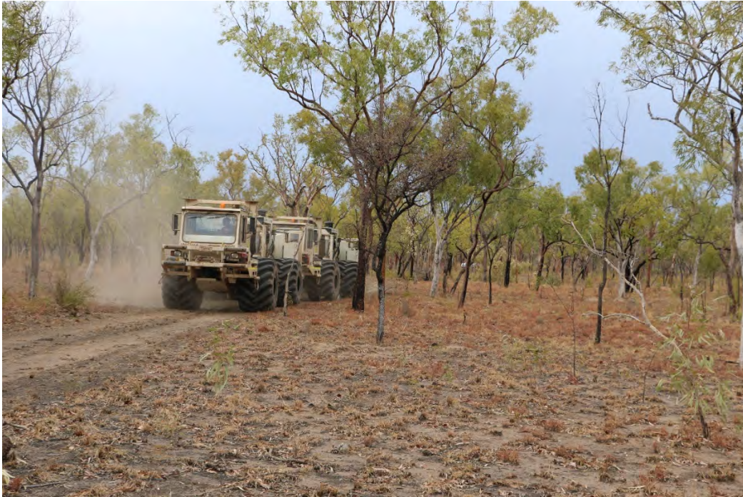
Figure 2.1: Two Seismic vibrator trucks working
