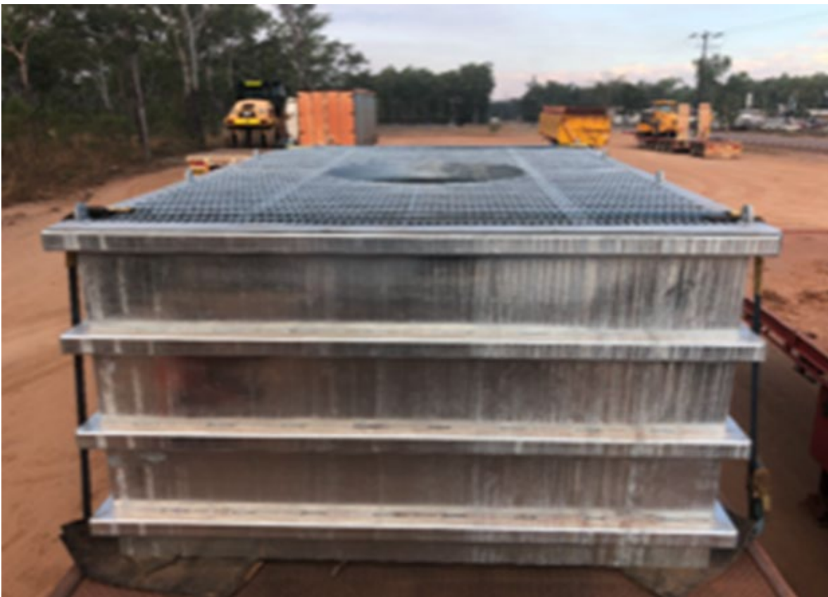
Figure 14: A cellar prior to installation
