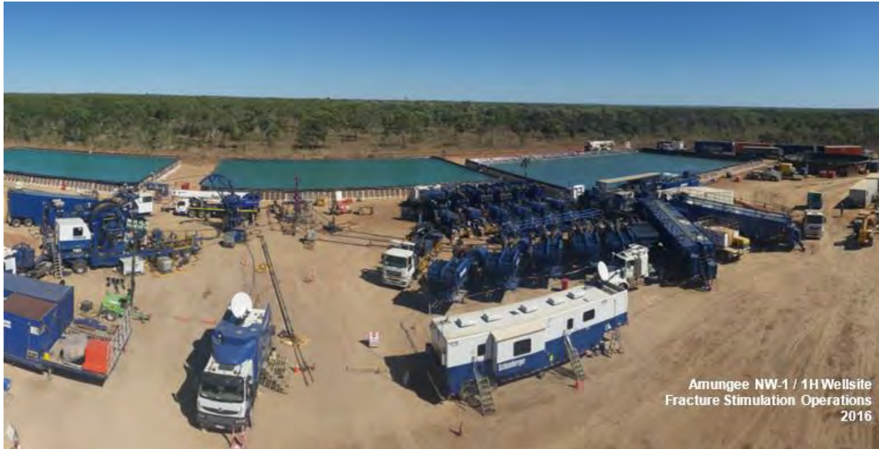
Figure 8: Example of stimulation lease layout.
