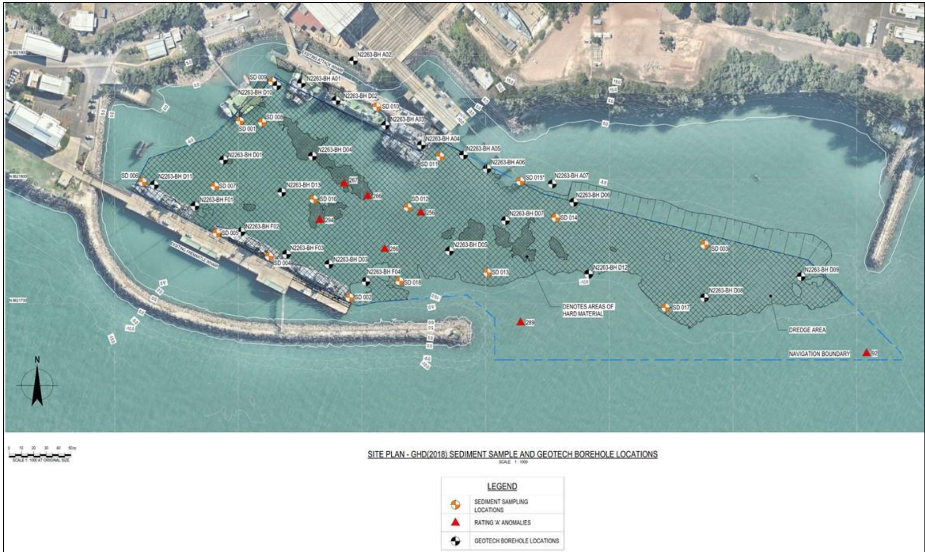
Figure 4.1 Current NCIS-5 Project Dredging Geotechnical Investigation Boreholes and Marine Sediment Sampling and Magnetic Anomaly Locations
