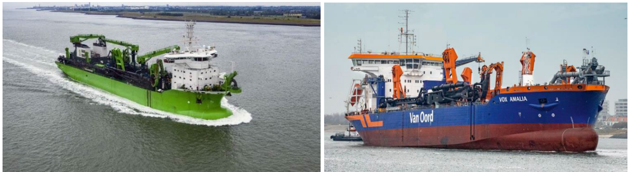
Figure 2-4: Trailing Suction Dredger's Bonny River (left) and Vox Amalia (right) (Allseas, 2022)
