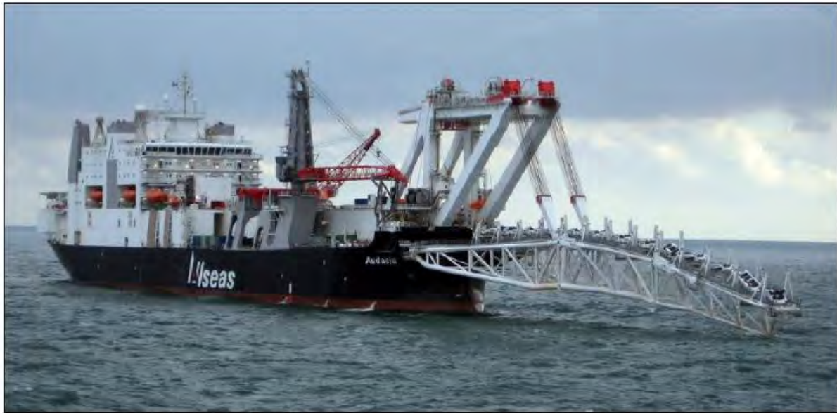
Figure 2-6: Deep water pipe lay vessel (Audacia)
