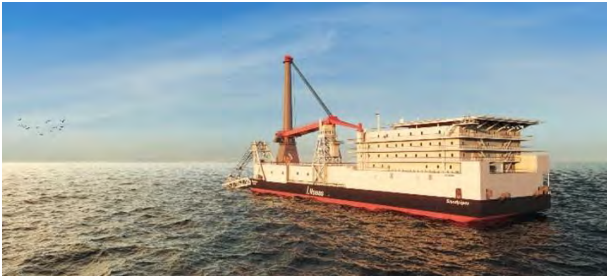
Figure 2-7: Nearshore pipe lay barge (Sandpiper)
