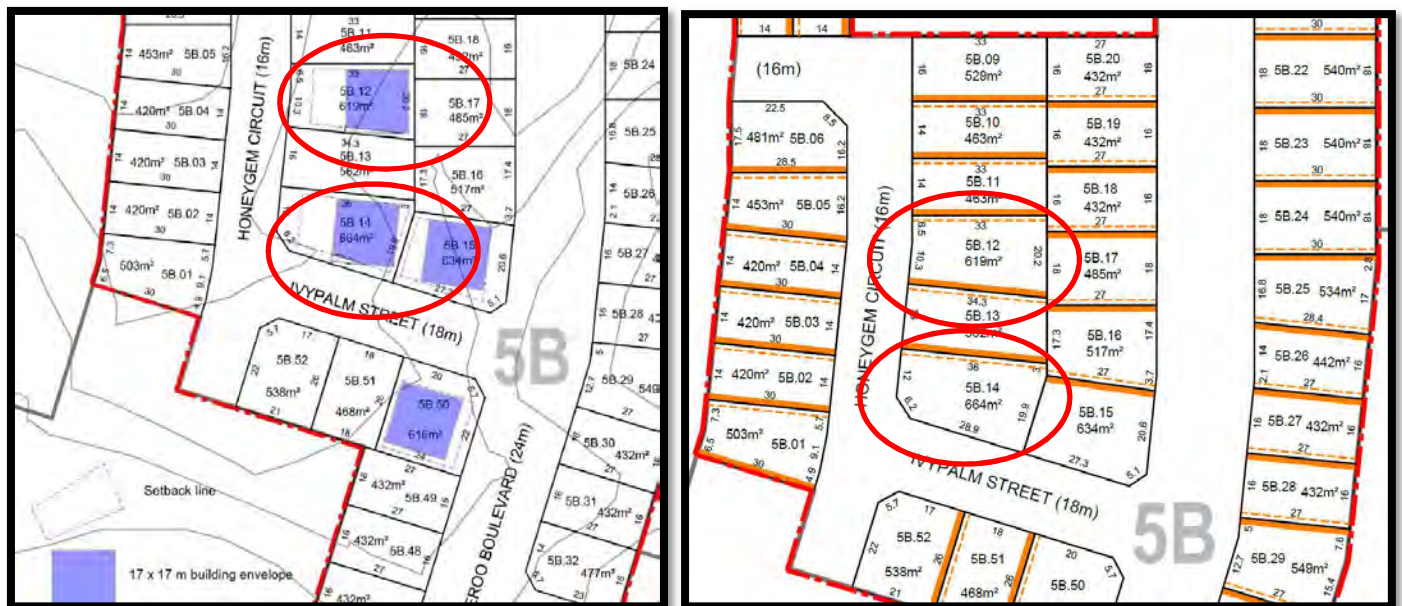
Figure 5: Proposed Lot 12 and 14 with non-compliant building envelopes.
