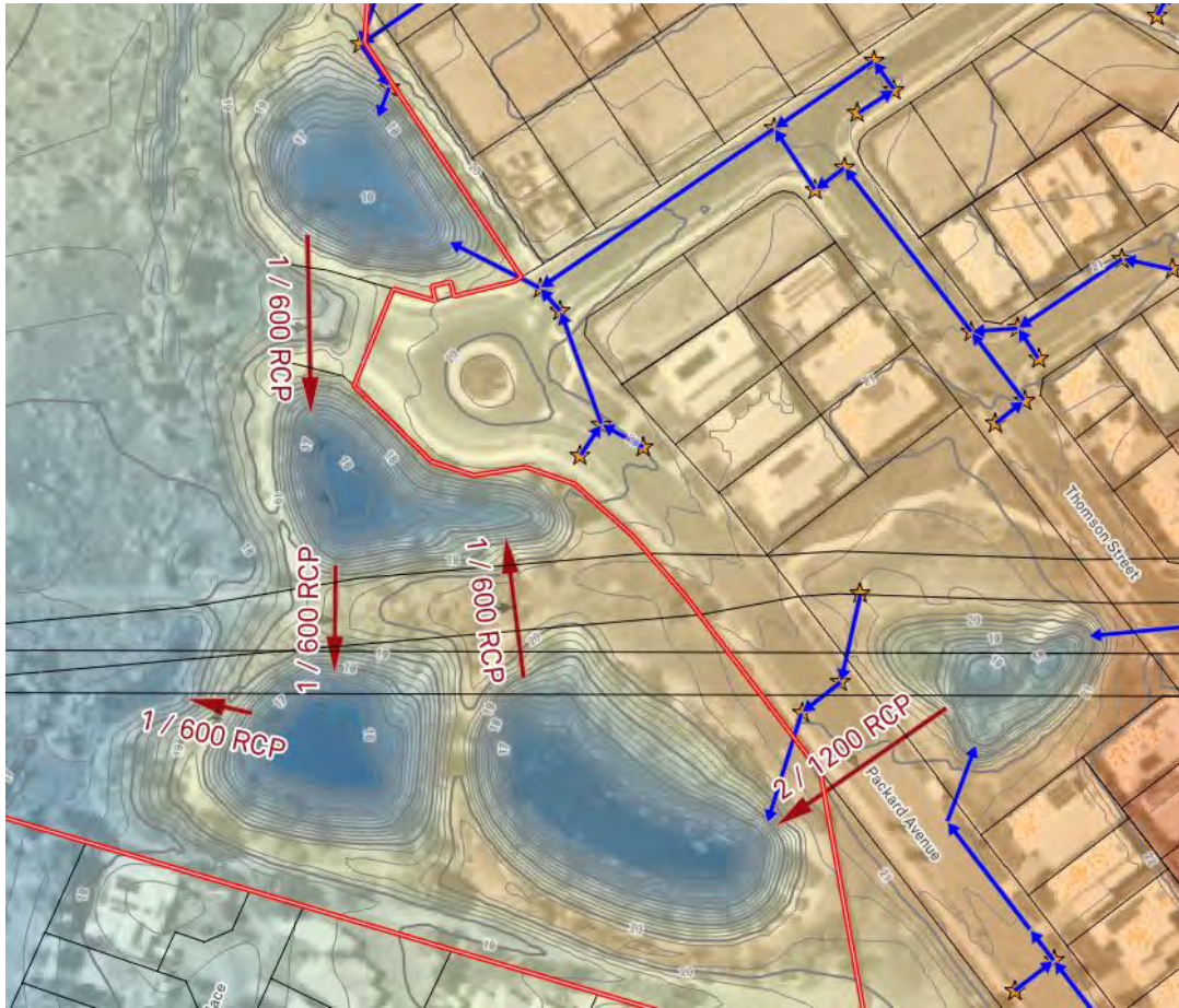
Figure 3-7 | Existing Hydraulic Structures – Ponds
