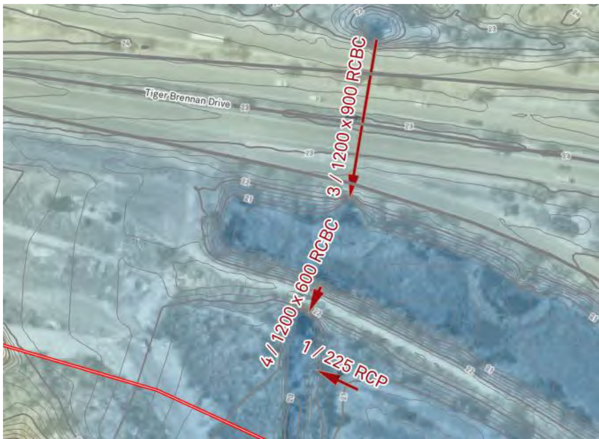
Figure 3-6 | Existing Hydraulic Structures – Tiger Brennan Drive
