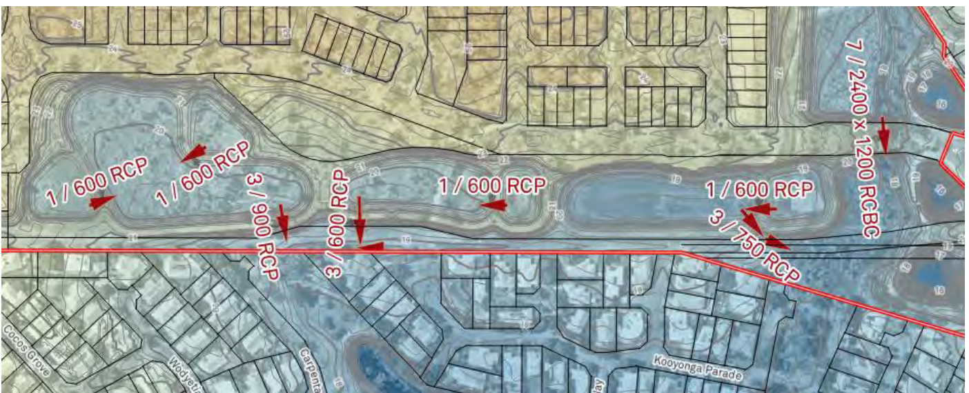
Figure 3-9 | Proposed Hydraulic Structures – Proposed Culverts
