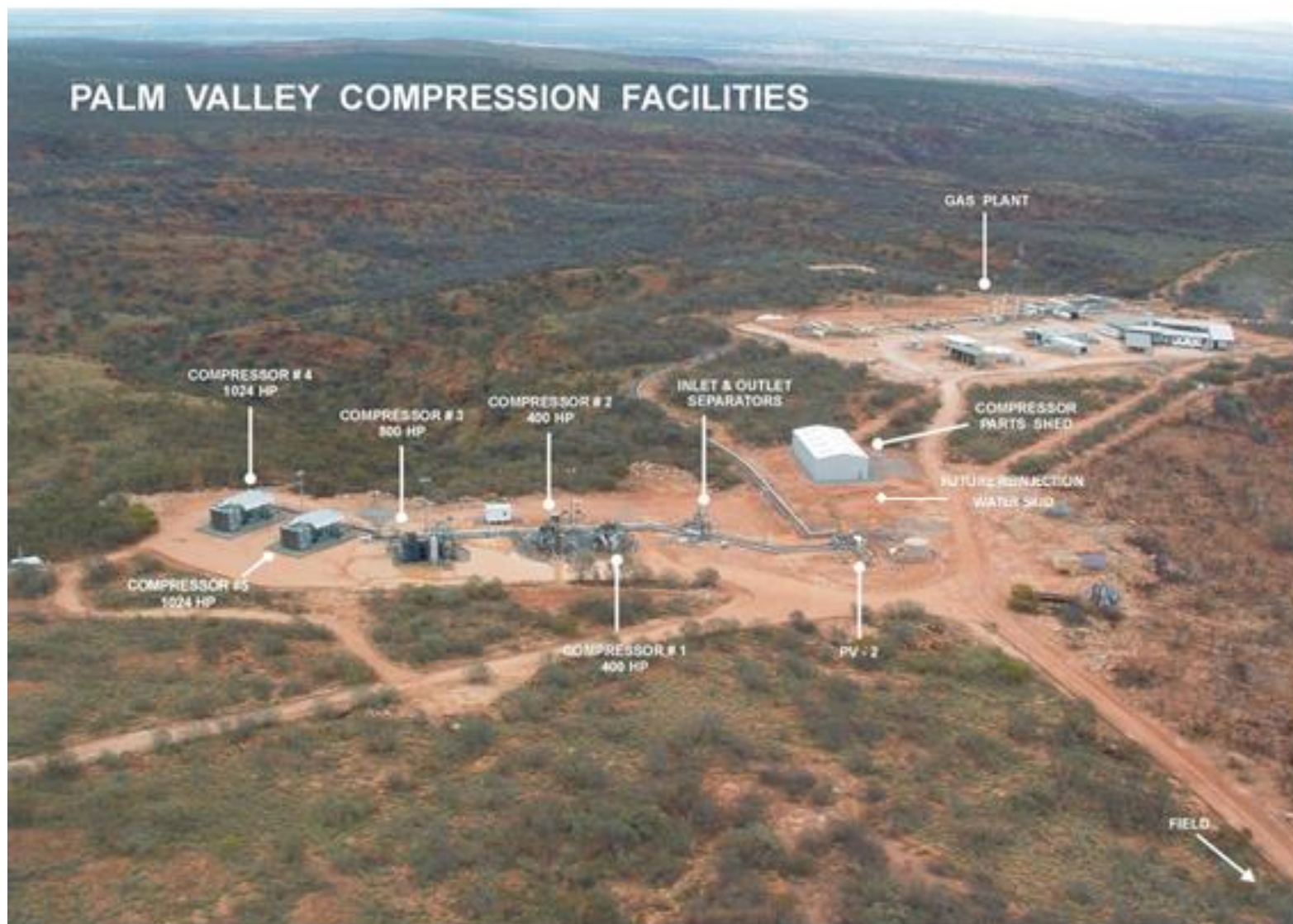
Figure 6-2 Annotated aerial image of the PVGF Central Compression Station
