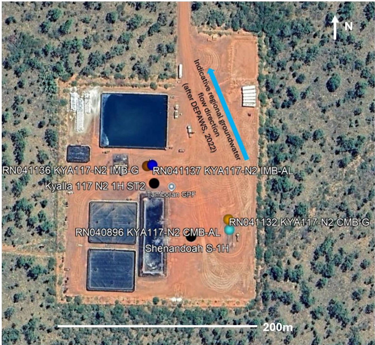
Figure 1 Kyalla 117 N2 site layout and indicative groundwater flow direction
