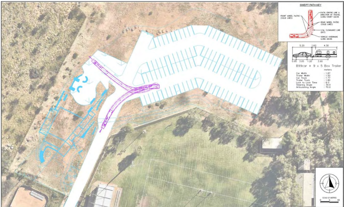
Figure 15: Food truck/trailer swept path
