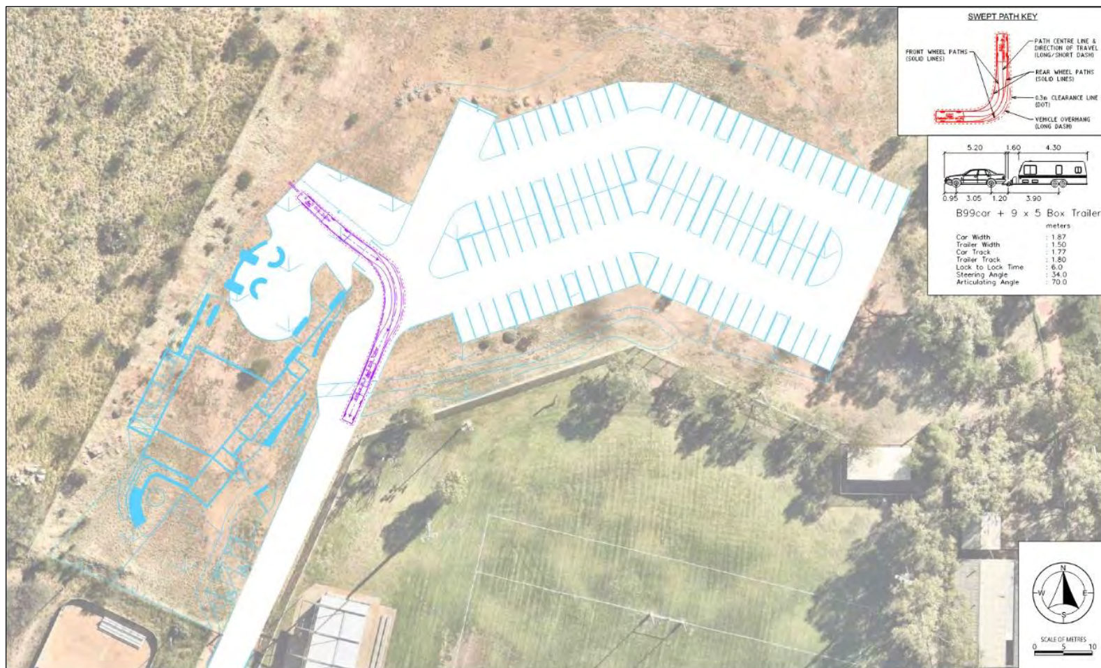
Figure 16: Food truck/trailer swept path
