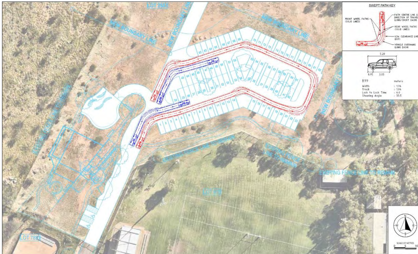
Figure 13: Design vehicle swept path – internal car circulation
