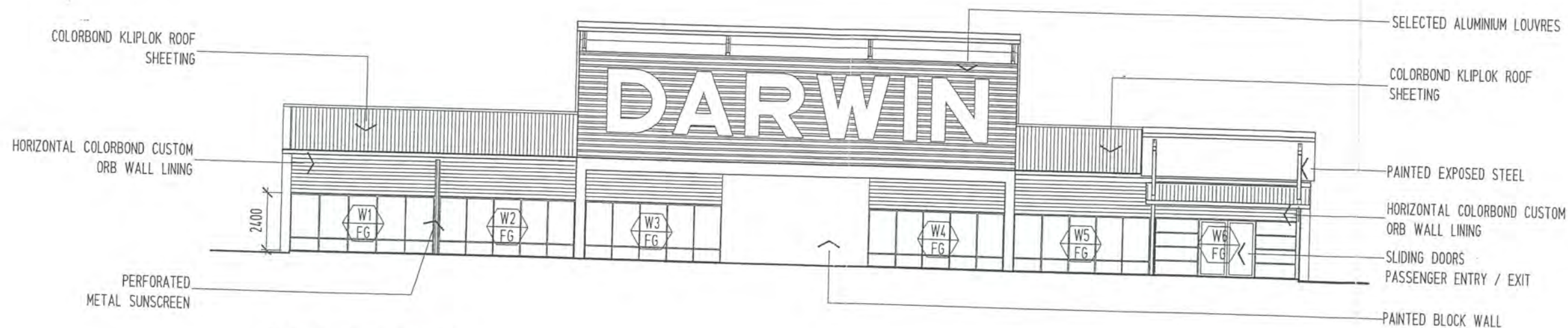
SOUTH ELEVATION SCALE 1 : 200
