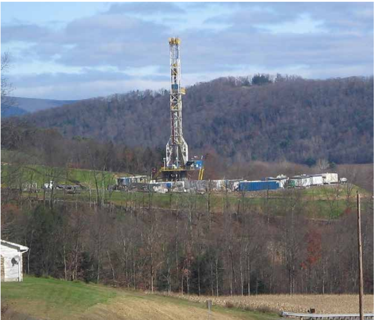
Figure 2: Tower for drilling horizontally into the Marcellus Shale Formation for natural gas in Lycoming County, Pennsylvania, USA
