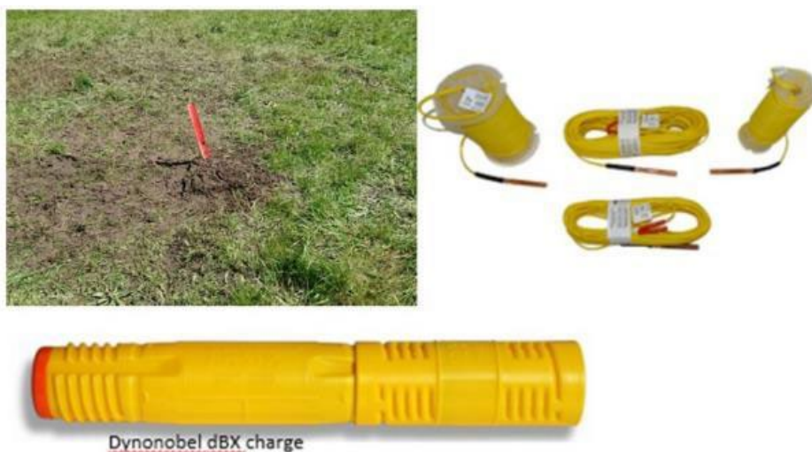
Figure 9: Example of loaded charge in hole ready for detonation and example of a charge used in dynamite seismic survey acquisition; charge length is approximately 400 – 500 mm
