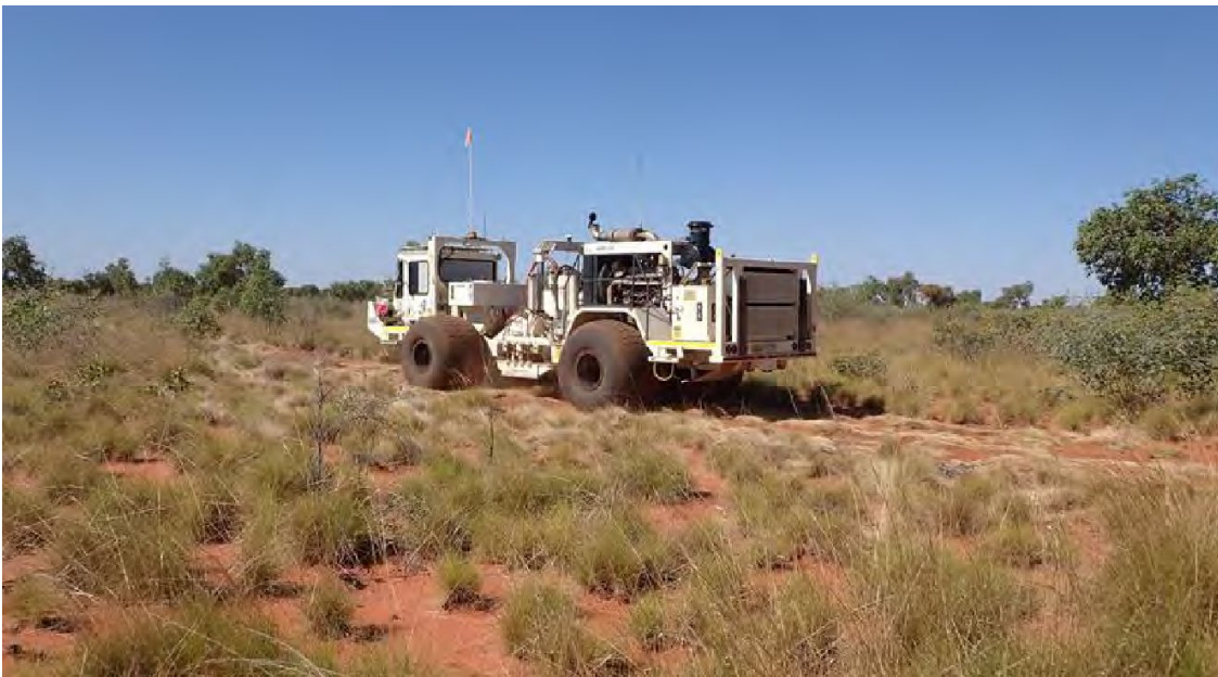
Figure 11: Example of a vibroseis truck used during seismic acquisition
