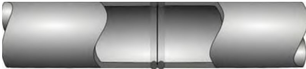
Figure 16: Standard butt fusion join (source: APGA, 2019)
