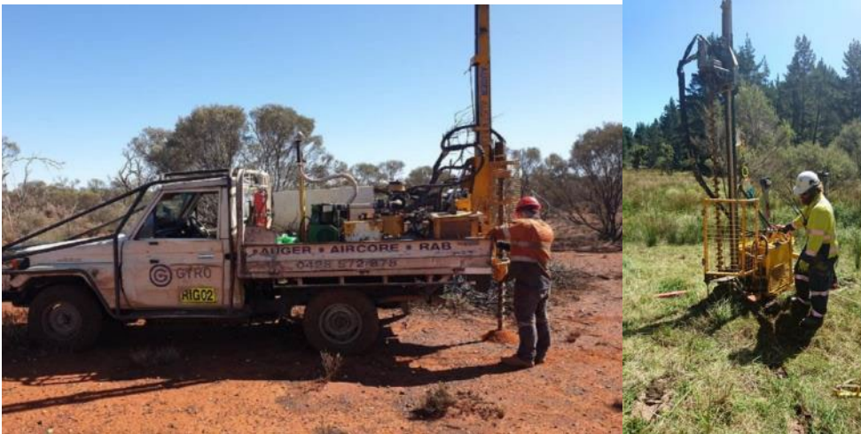
Figure 8: Example of a small rig that could be used for installing dynamite charges during a seismic survey
