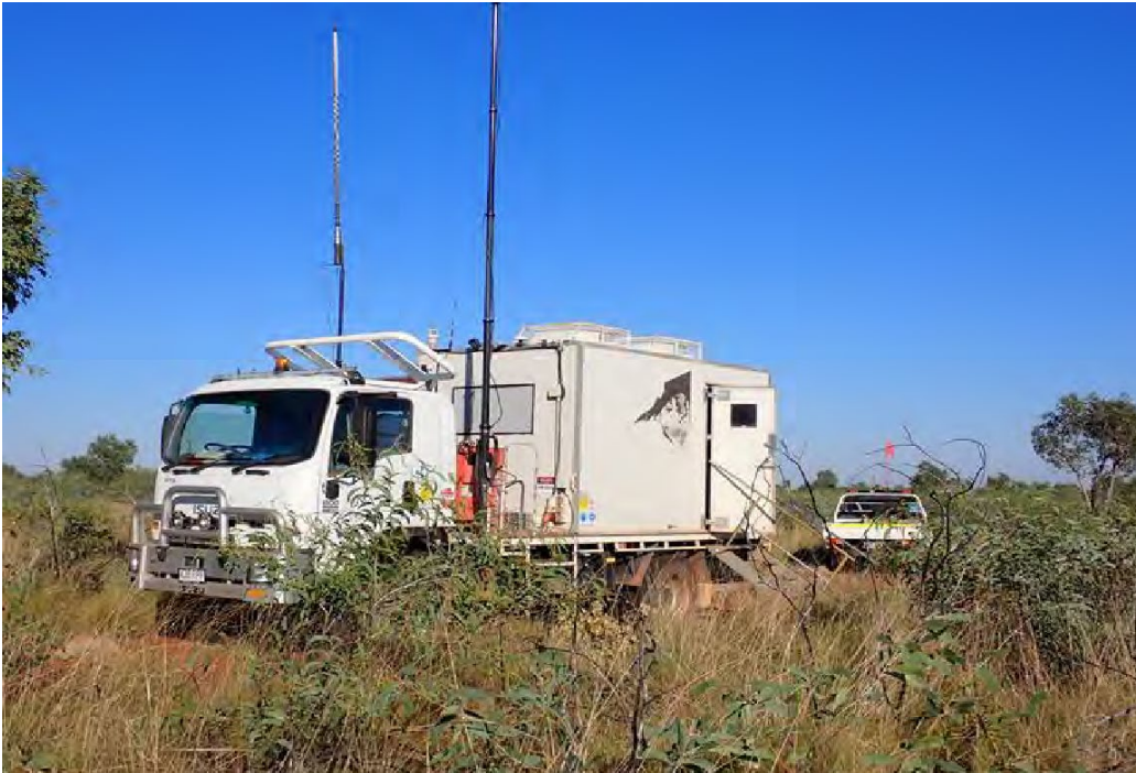
Figure 12: Data recording van used during seismic acquisition
