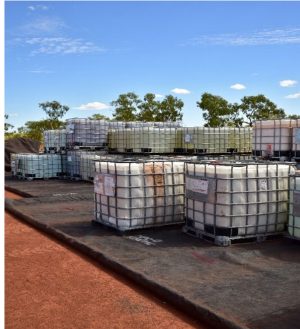
Figure 59: Examples of spill mats used to contain potential wastewater transfer spills
