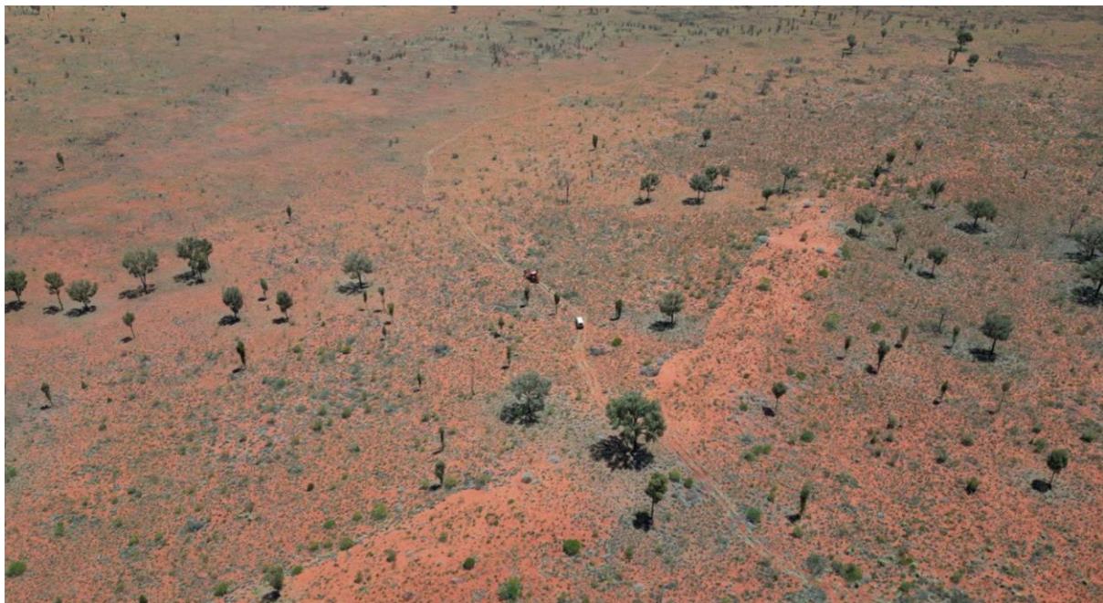
Figure 12: Line weave through existing vegetation clearances in the Amadeus Basin
