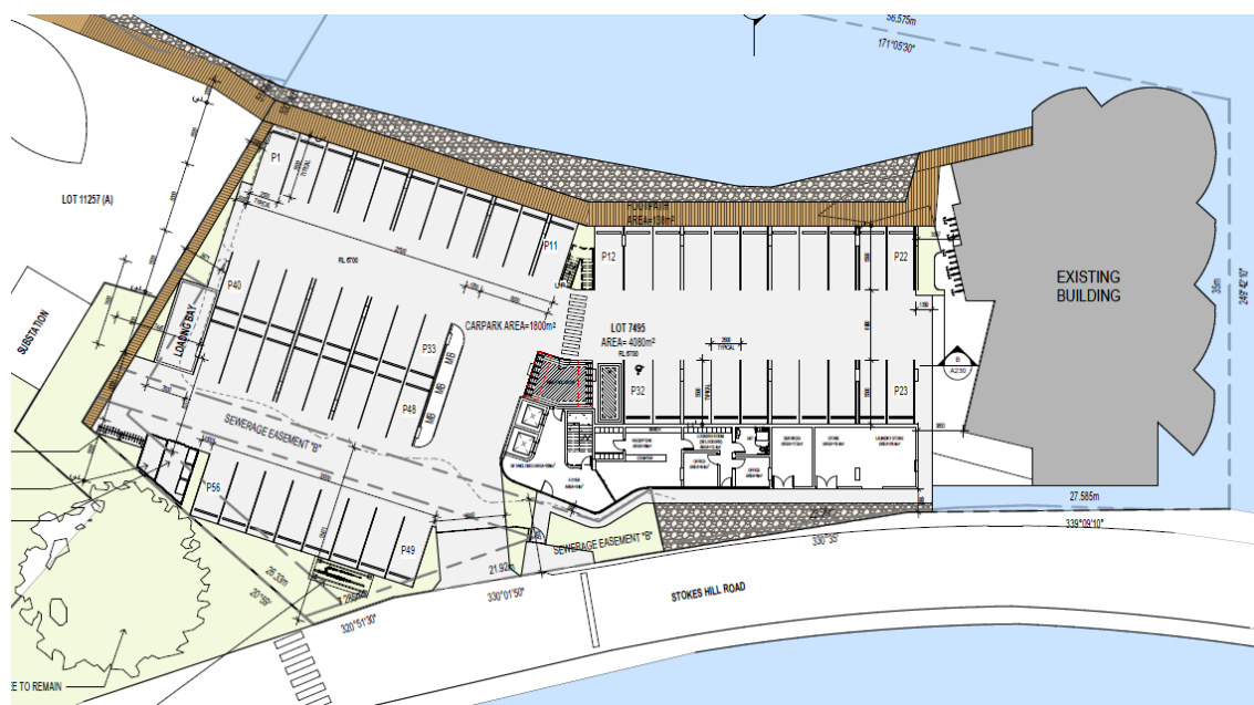
Figure 9: Proposed development – Ground level car park
