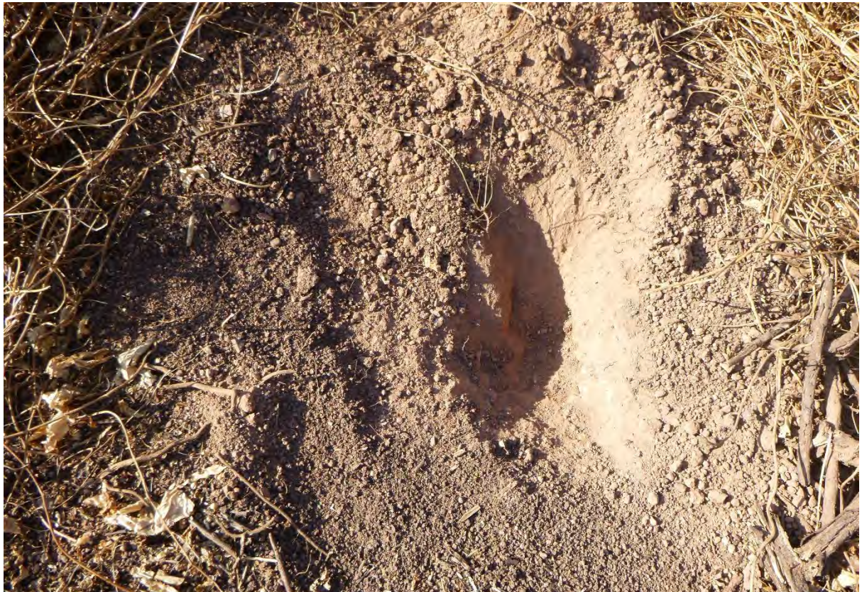
Figure 7 Land type B Soil - Shallow (0.3m), moderately well drained, gravelly brown Kandosol
