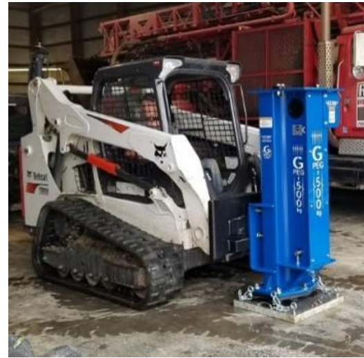
Figure 3.5-14 Indicative weight drop unit on skid steer
