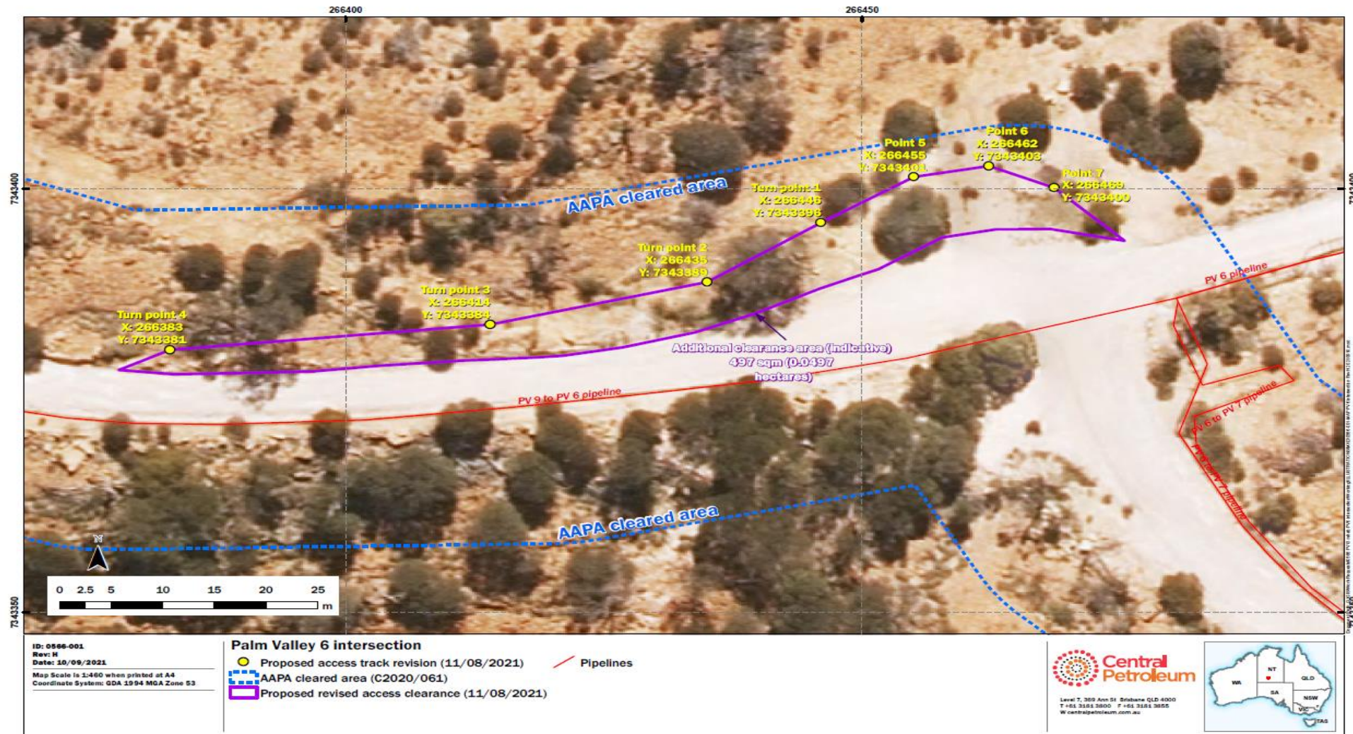
Fig 1: The Road requires widening to permit a large drilling rig and trailers to negotiate the PV6 – PV7 road junction and avoid existing pipeline infrastructure. Point numbers are described in Table 1.
