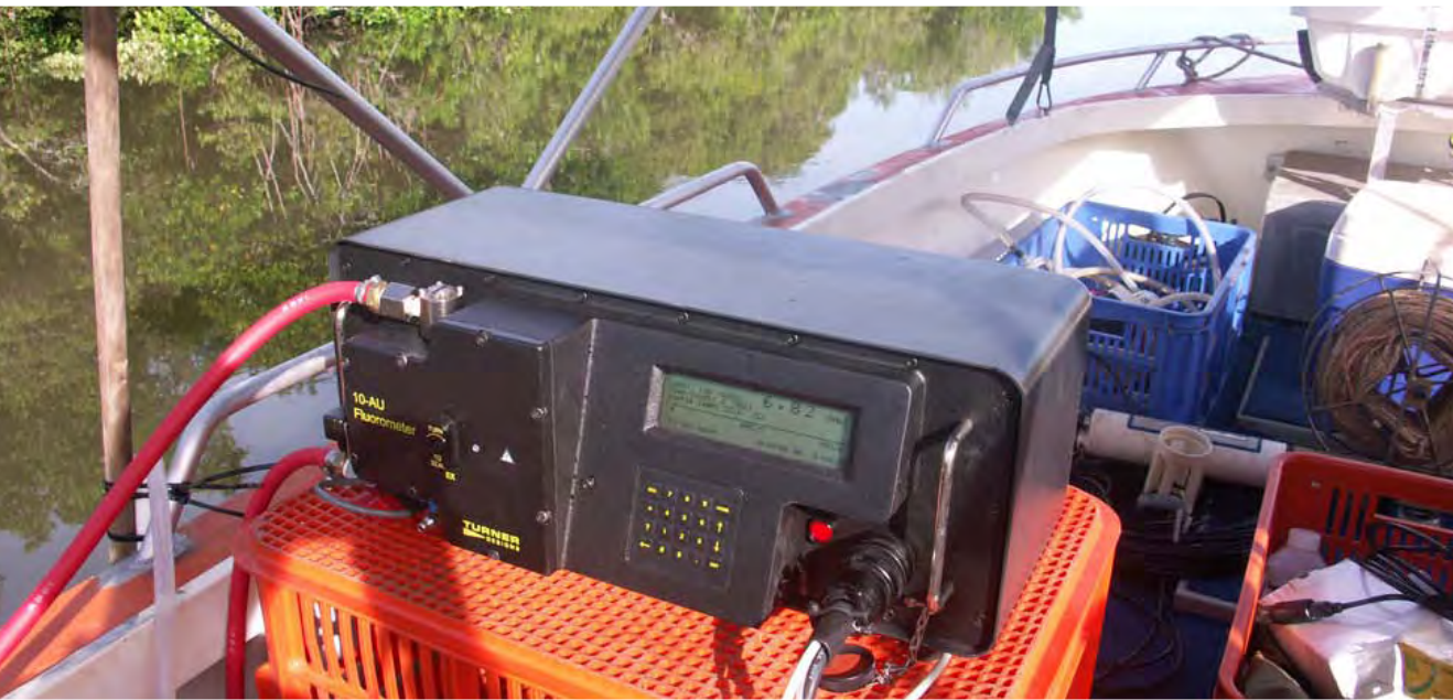
A fluorometer is used to gather data for chlorophyll a mapping.
