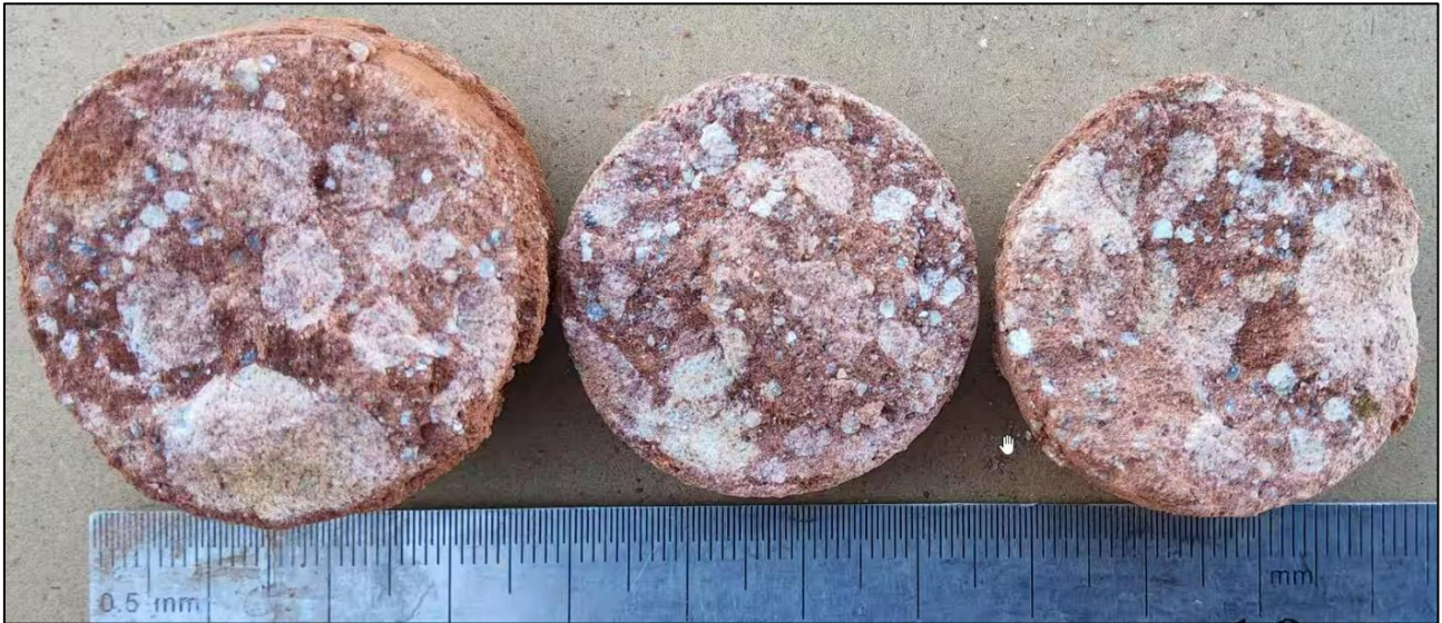
Figure 5: Borehole BH02, SPT sample at 3.0m, showing laterised conglomerate, logged as 'extremely weathered material'.
