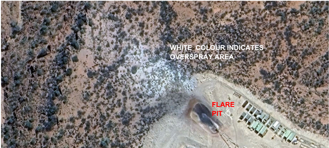
Figure 2: Google earth image of flare pit overspray (imagery date: 10 December 2022)
