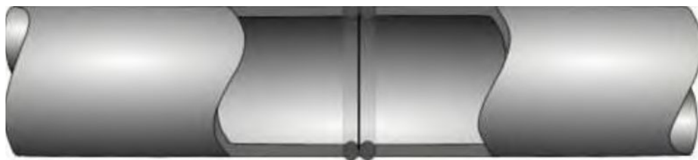
Figure 19: Standard butt fusion joint (source: APGA, 2019)
