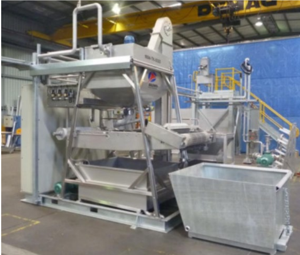
Figure 16: Example of a fully automated, skid mounted water treatment package / system, which will be located in the SPCF under cover (source: Baldwin Industrial Systems 2024 )
