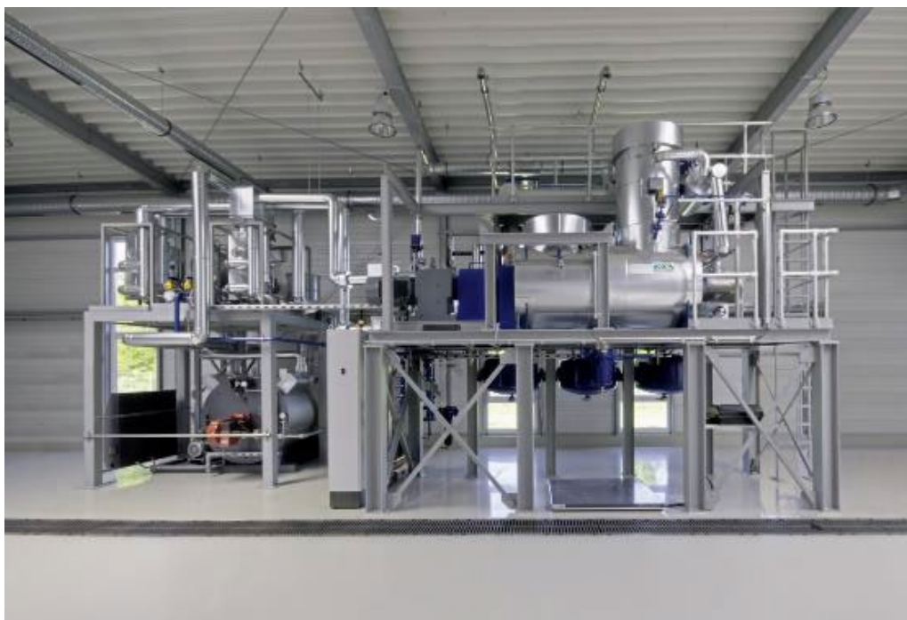
Figure 18: Example of a mercury removal unit, designed to be skid mounted ( encon industries, n.d. )
