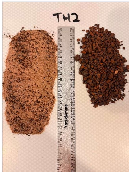
Photo 26: Composition of TH2 sample following sieve analysis (gravel and sand only)
