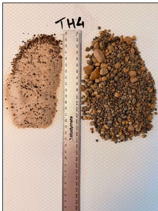
Photo 28: Composition of TH4 sample following sieve analysis (gravel and sand only)
