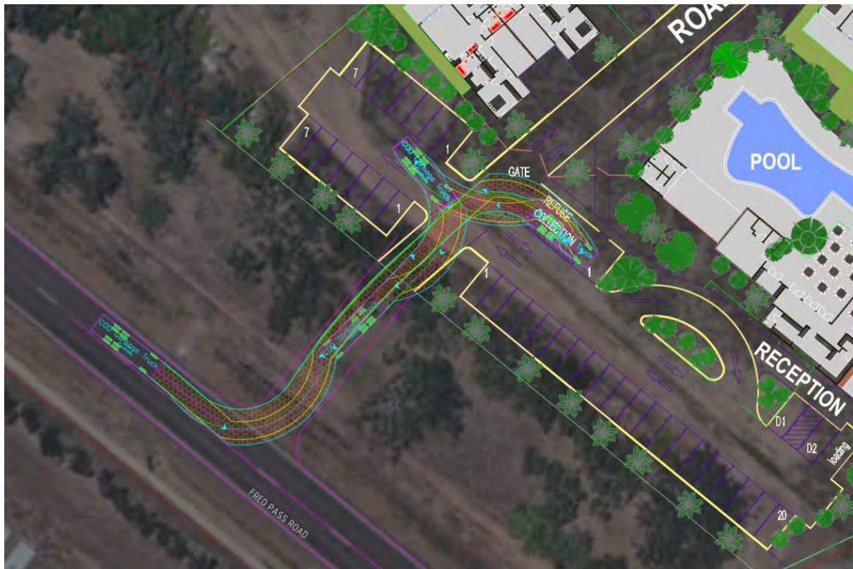
Figure 4 Refuse Vehicle Swept Path
