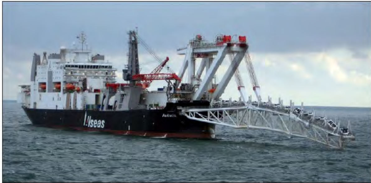
Figure 2-6: Deep water pipe lay vessel ( Audacia )
