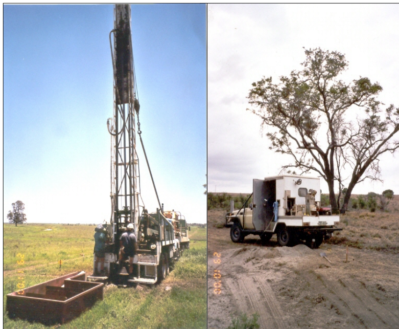
Figure 6: Up hole drilling rig and LVL recording truck
