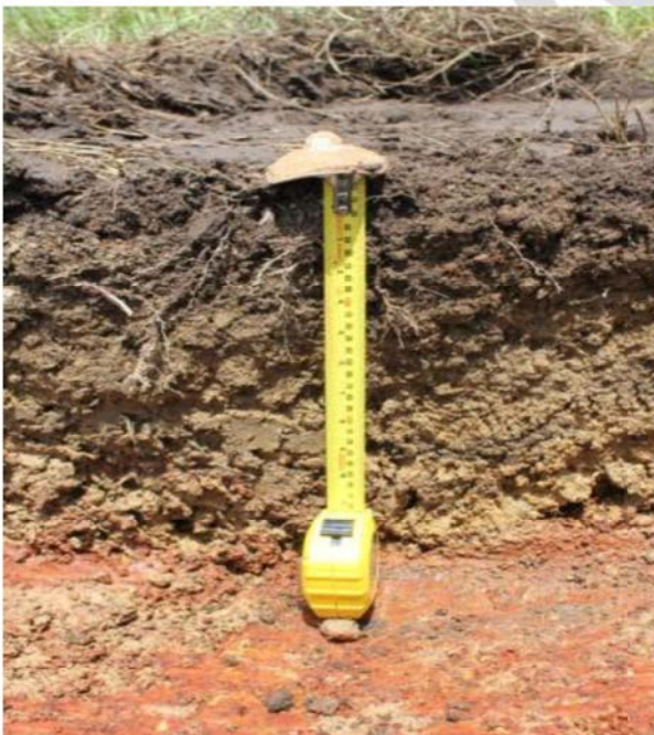
Figure 11 Test Pit 8: Very shallow soil profile in the SW of the property
