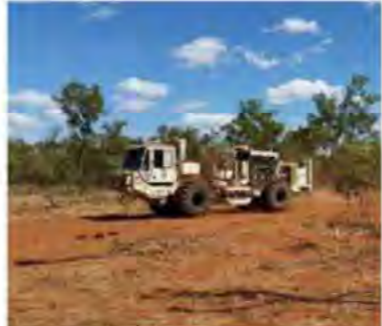
Plate 2 Inova AHV-IV "Renegade" seismic vibrator
