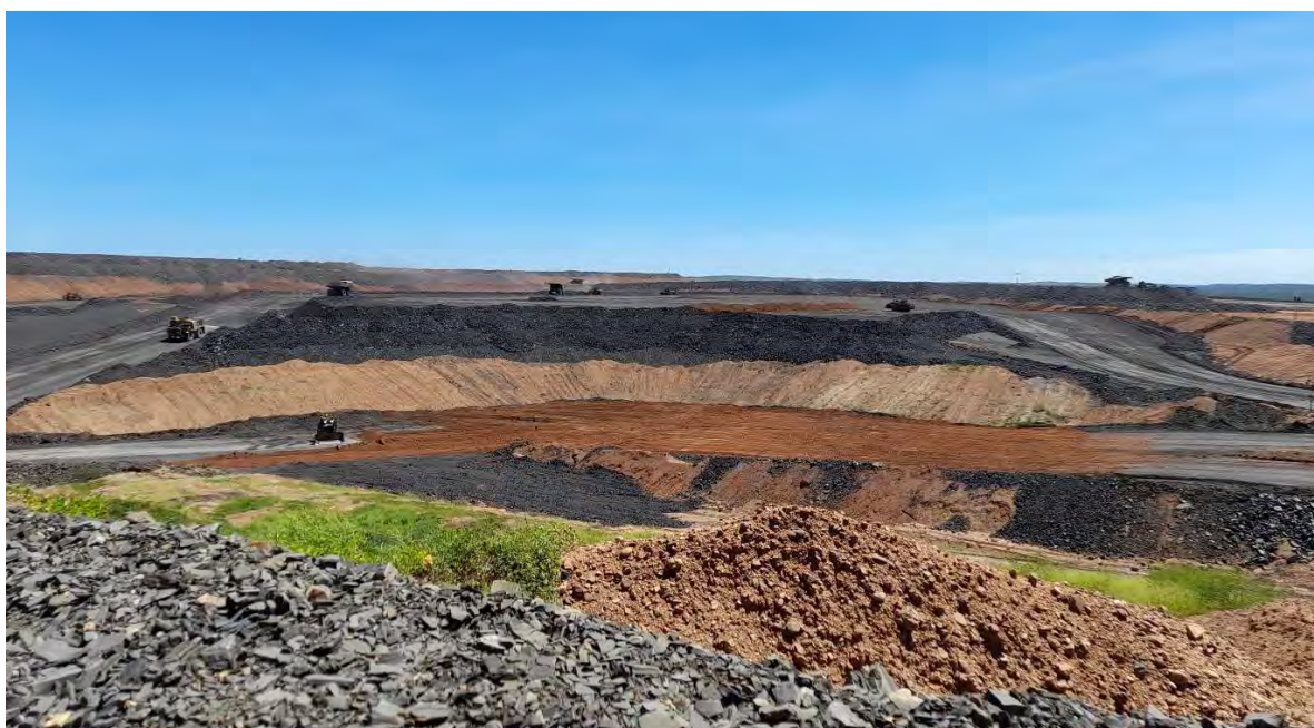
Photo 4-1: Active working face showing construction of a PAF (RE) cell (David Jones, April 16, 2025)
