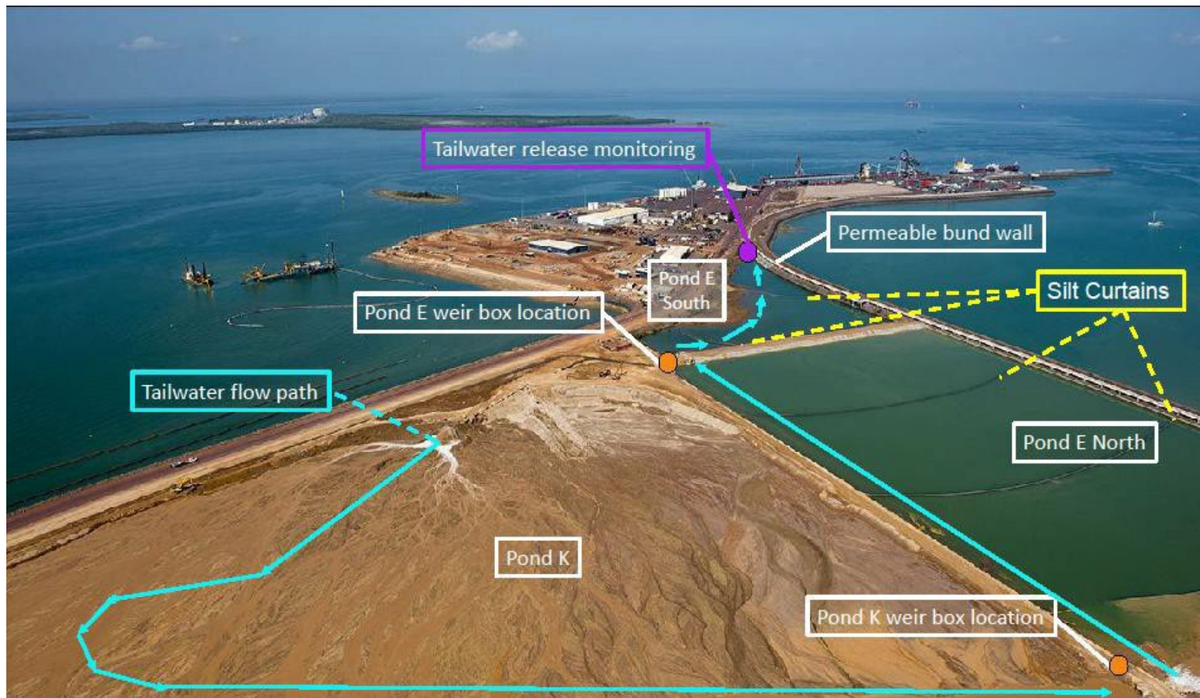
Figure 9 Indicative settling pond configuration
